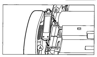
Open the top cover, then open the front lid by sliding the lever towards you.
